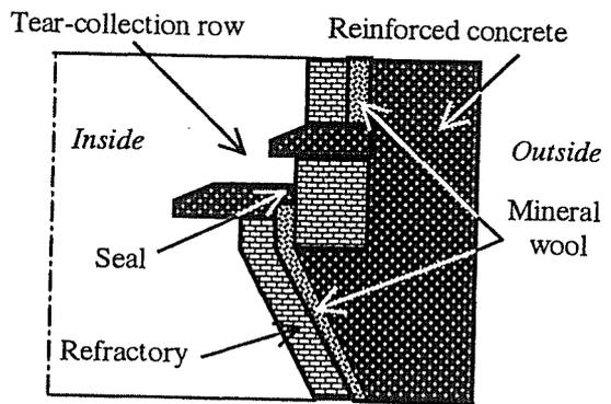
Fig. 1. Typical design of a reinforced concrete smokestack
