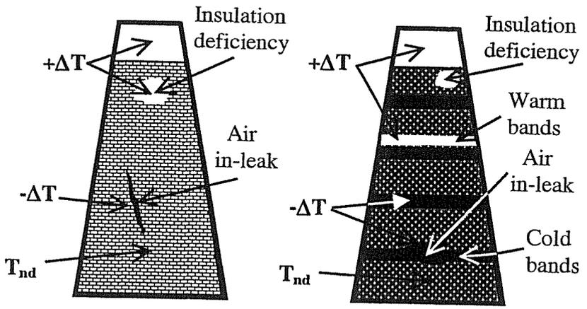
Fig. 2. Schematic presentation of typical smokestack thermograms:
