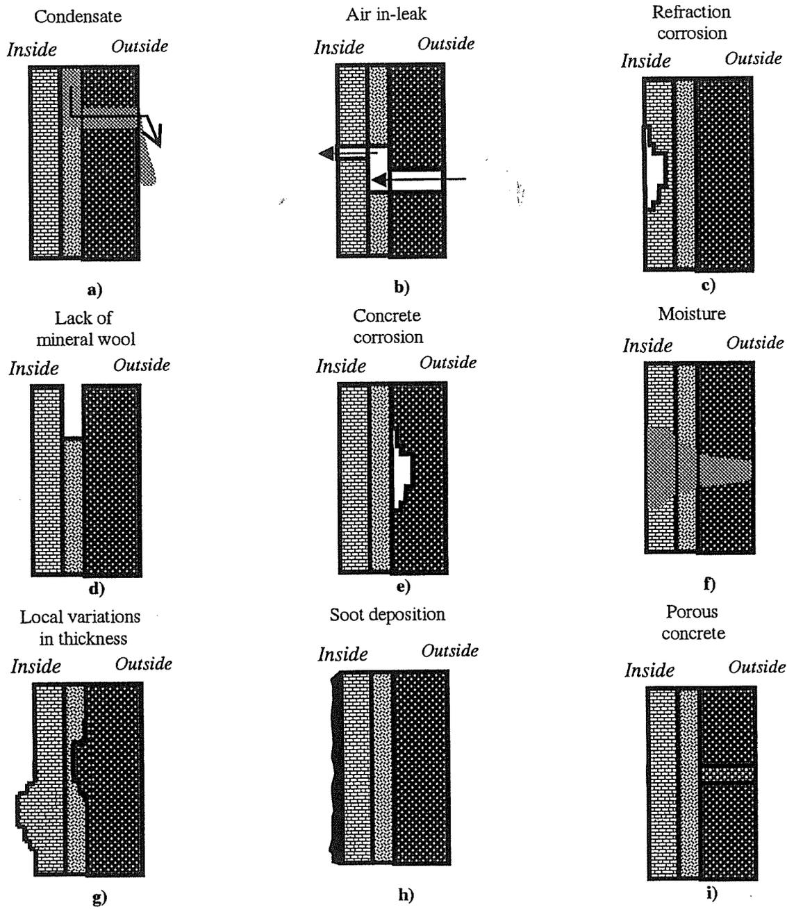
Fig. 3. Smokestack defect models
